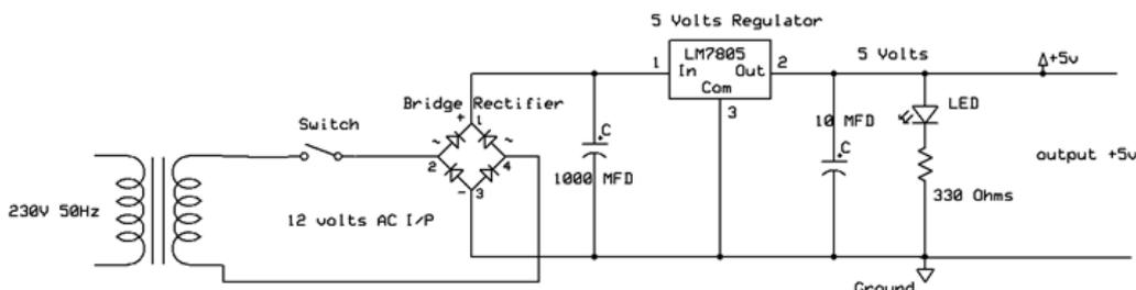
Fig:2.3.1 Circuit Diagram Of Regulated Power Supply
