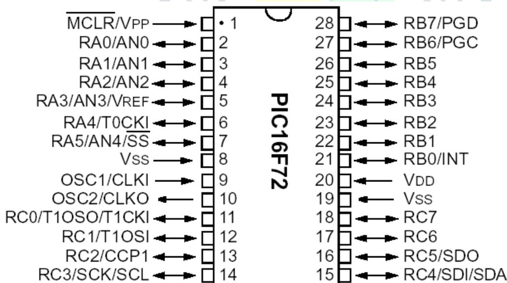
**Fig. 2.2.1 Pin Description of PIC16F72**
