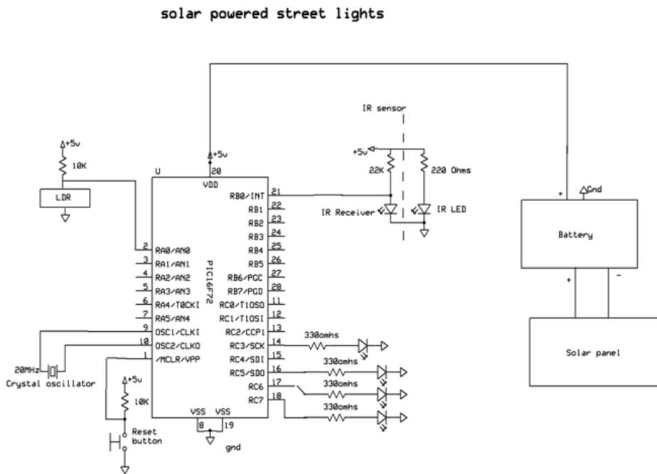
Fig: 2.2.4 Circuit Diagram of Solar Power Street Lights
