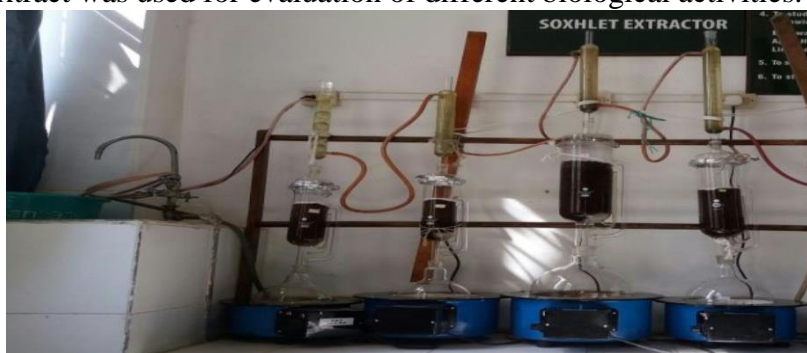
Fig2: Extraction of plants by using Soxhlet's apparatus
