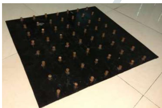
Fig. 6 Absorber plate with copper fins.[slb1]
