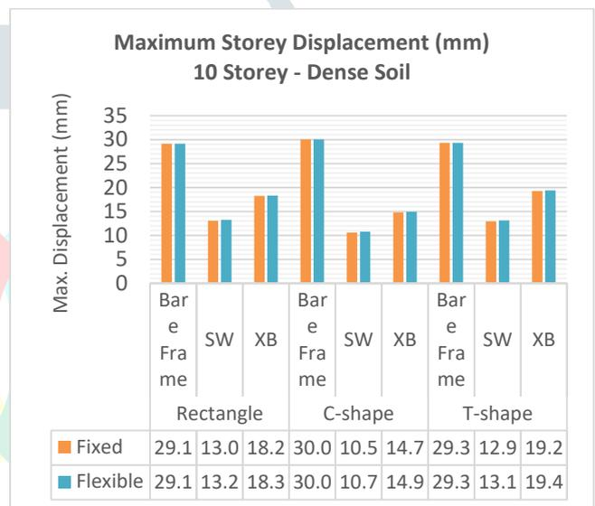
Maximum Storey Displacement (mm) of 10 Storey: (a) Rock (b) Dense Soil
