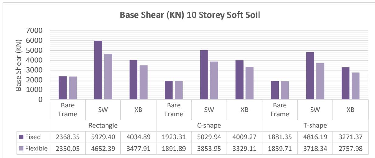
Base Shear (KN) for 10 Storey at Soft Soil
