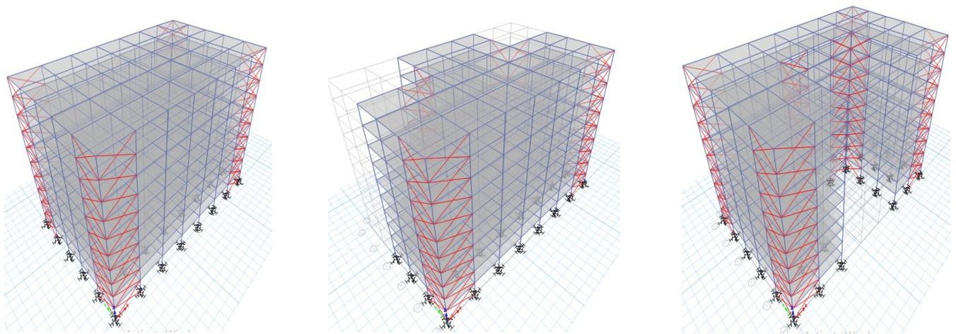
Fig 2. Elevation view of 10 storey having X-bracing (a) Rectangle (b) T-shaped (c) C-shaped
