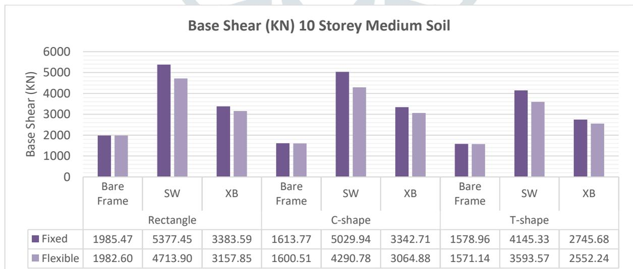
Base Shear (KN) for 10 Storey at Medium Soil
