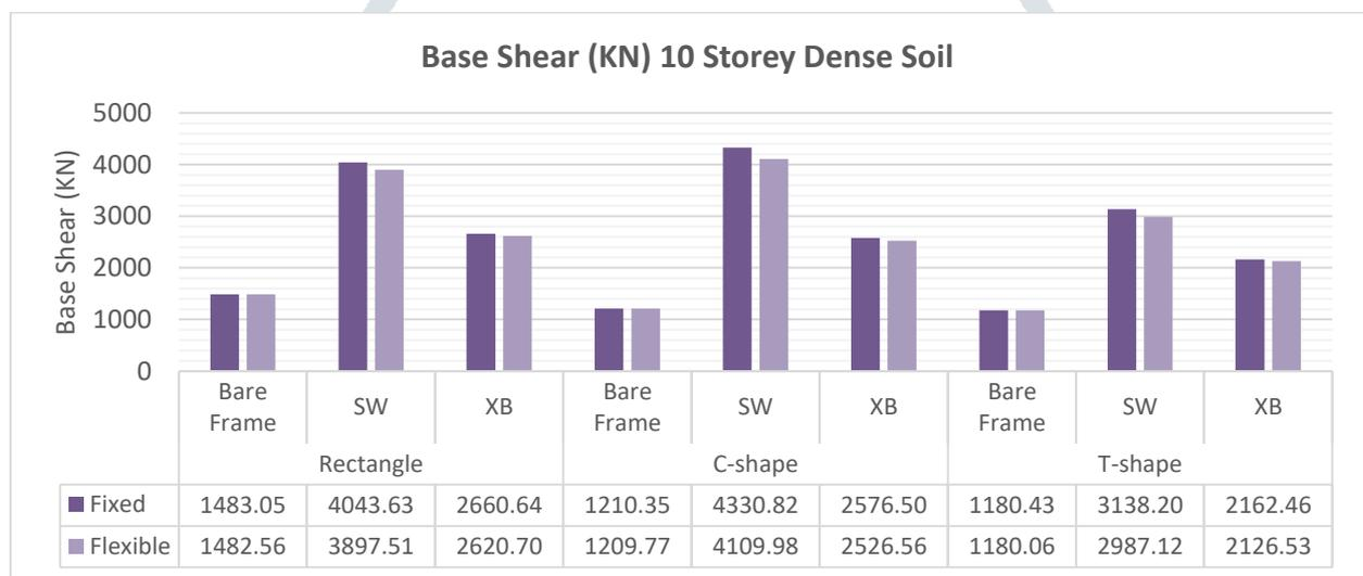
Base Shear (KN) for 10 Storey at Dense Soil
