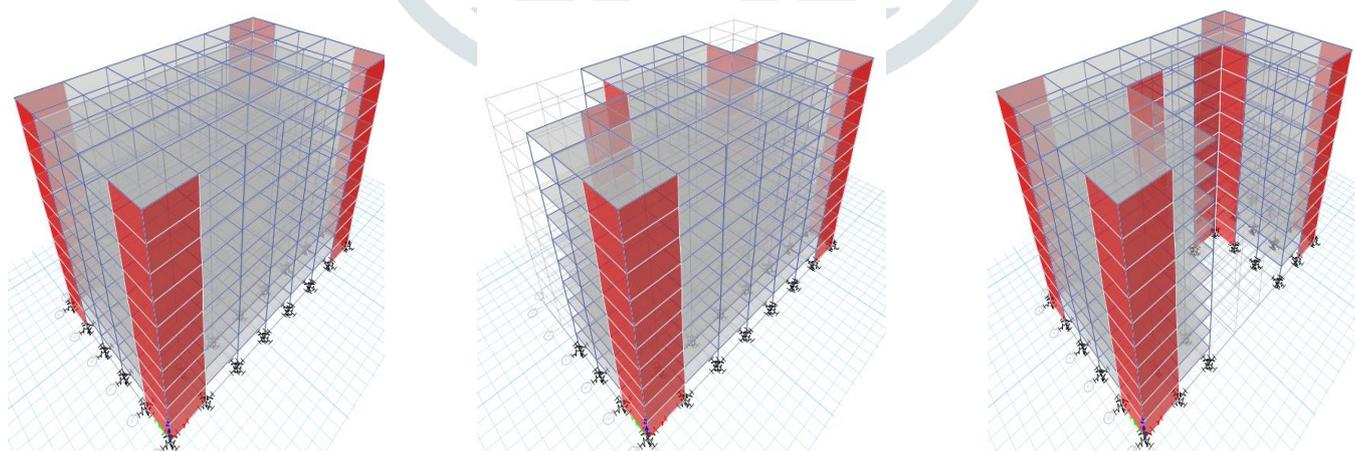
Fig 1. Elevation view of 10 storey having shear wall (a) Rectangle (b) T-shaped (c) C-shaped
