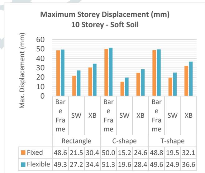
Maximum Storey Displacement (mm) of 10 Storey: (a) Medium Soil (b) Soft Soil
