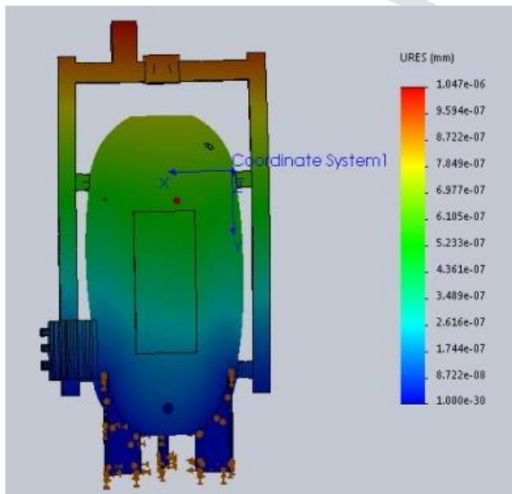
Fig.11.a. displacement Analysis.
