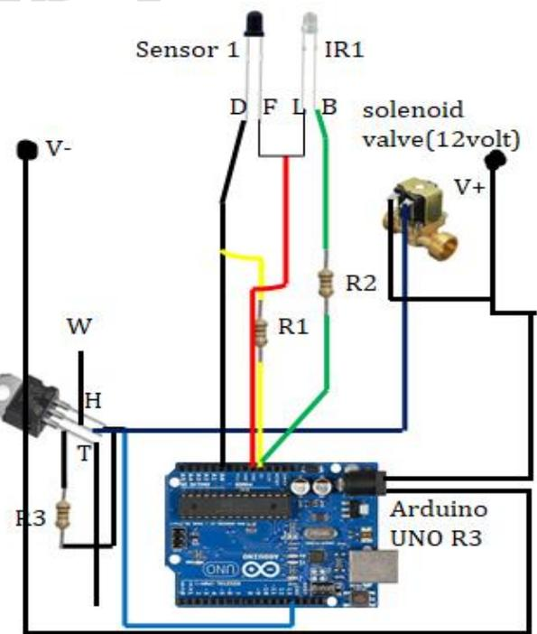
Fig.9. System of position detector sensor.
