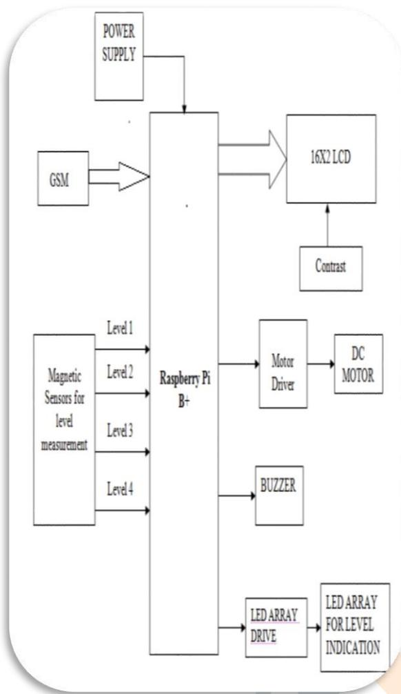
The water level at distinctive level is sensed through which the gate is closed or open. That is while the water is rises to level 3 the closed dam shutter is completely opened, for stage 2 gate is partly closed at the same time as for stage 1 the gate is absolutely closed. Dams are generally built with a drain or similar mechanism to govern water stages in an impoundment for normal maintenance or emergency purposes.
