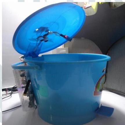
**Figure 7: Bin open with the ultrasonic sensor and the humidity sensor**
