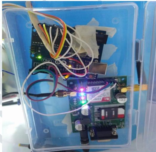
Figure 4: The GSM module and the Arduino board.
