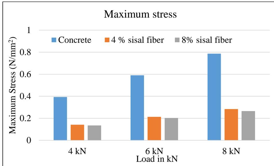
Figure 2 Effect of addition of the sisal fiber on the maximum stress
