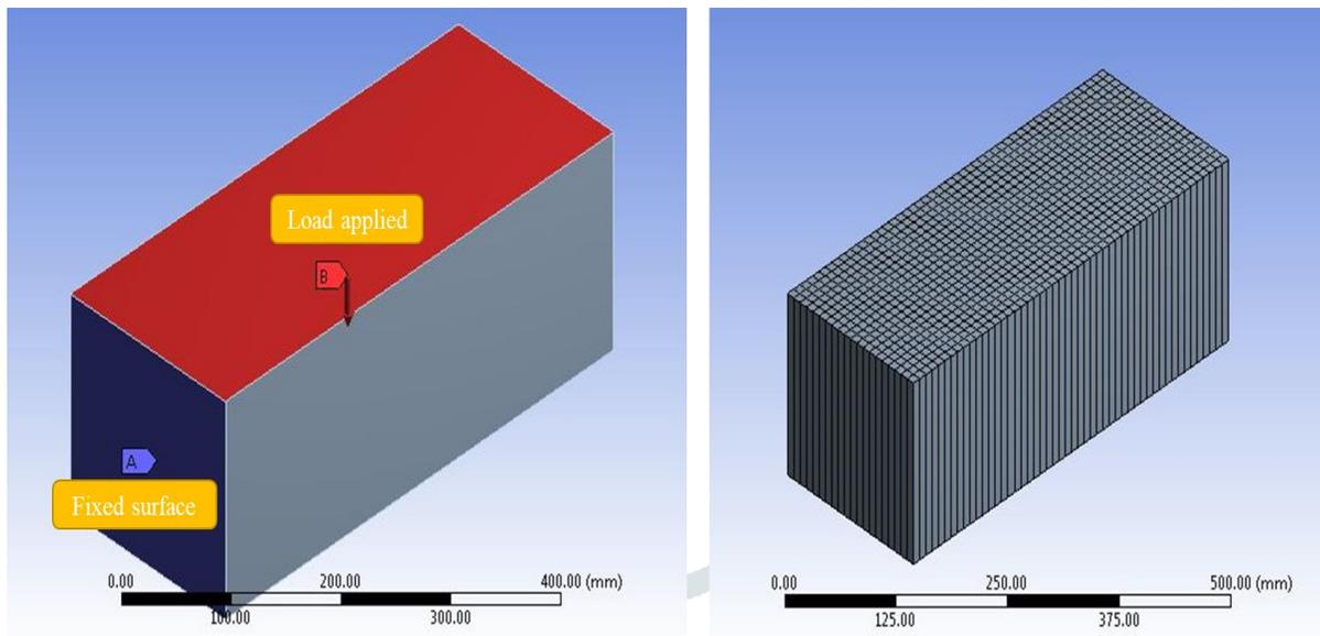
Figure 4.2 Boundary conditions and the mesh model used for the analysis.
