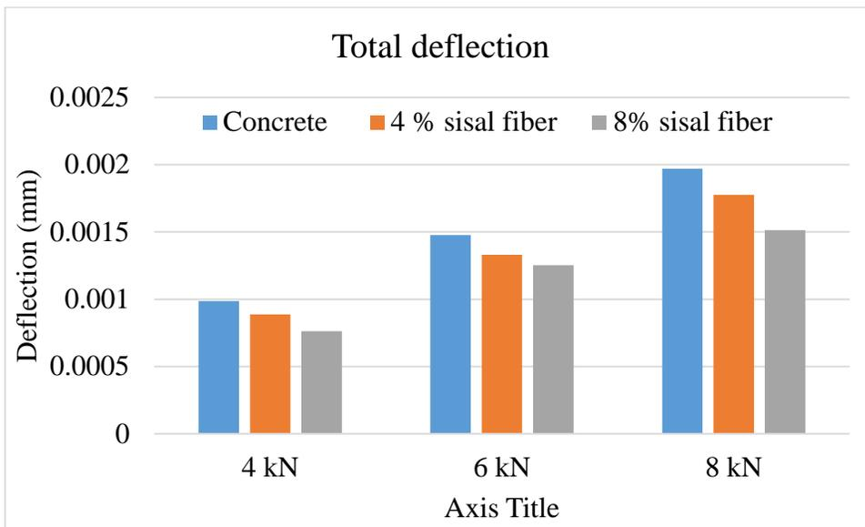
Figure 4 Effect of addition of the sisal fiber on the total deflection.
