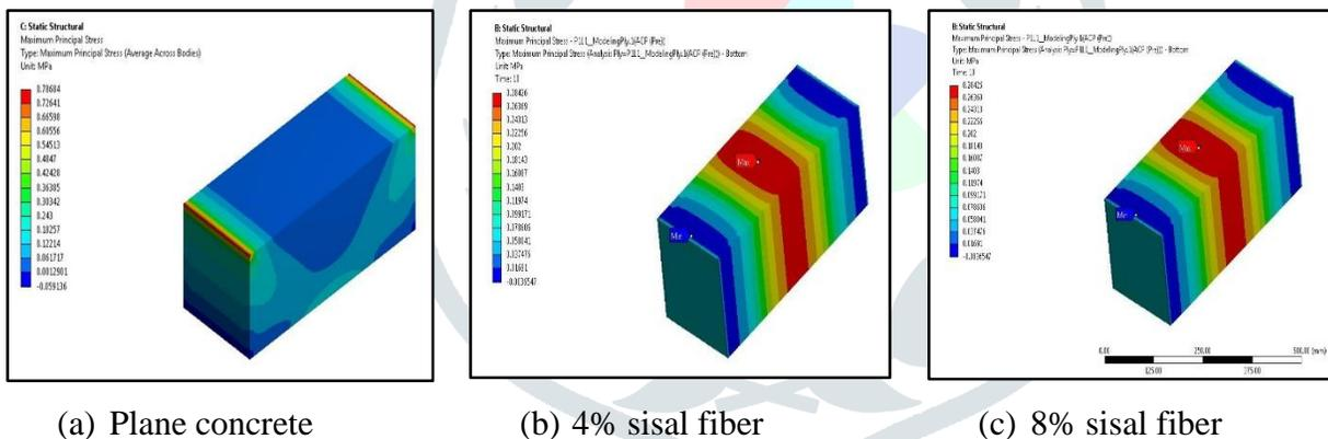
Figure 3 Effect of addition of sisal fiber on maximum principal stress
