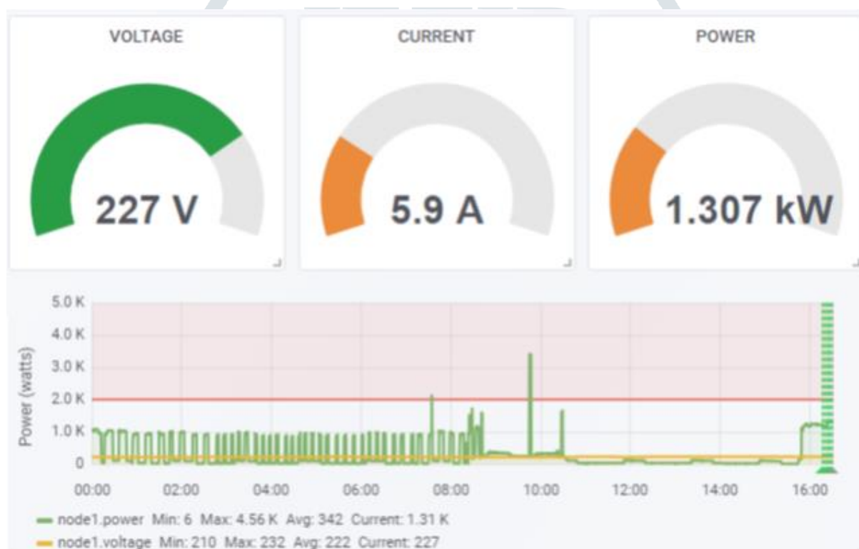
figure 8.3.1 the dashboard of the developed energy monitoring system.
