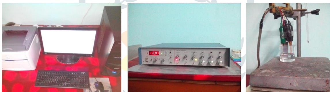
Fig. 1 The instrumental set-up of the three electrodes cell connected with the potentiostat/galvanostat via transducer with winDaq software installed computer system.
