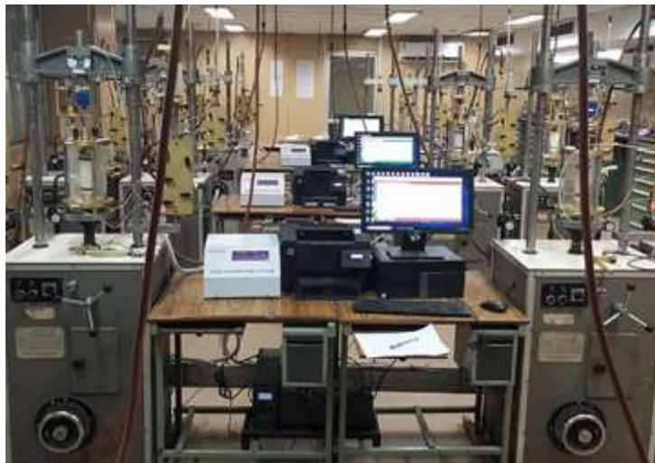
Fig. 5. Semi-automatic triaxial machine setup
