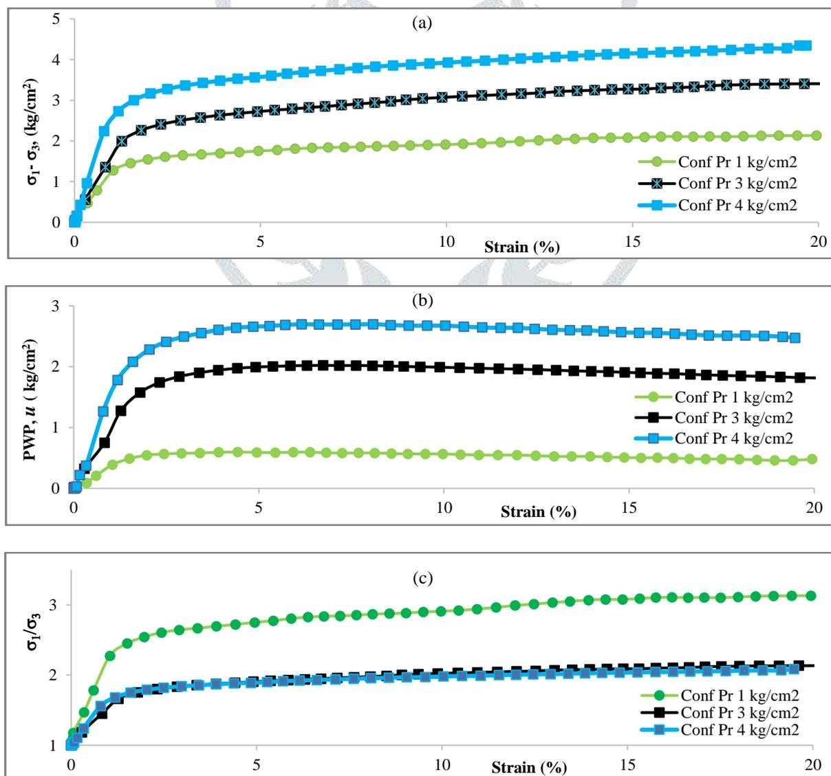
Fig. 7. (a) Deviator stress ( $\sigma_d$ ) - strain (%) graph, (b) Pore water pressure (u)-strain (%) graph and (c) Stress ratio ( $\sigma_1/\sigma_3$ ) -strain (%) graph for sample no. 1.
