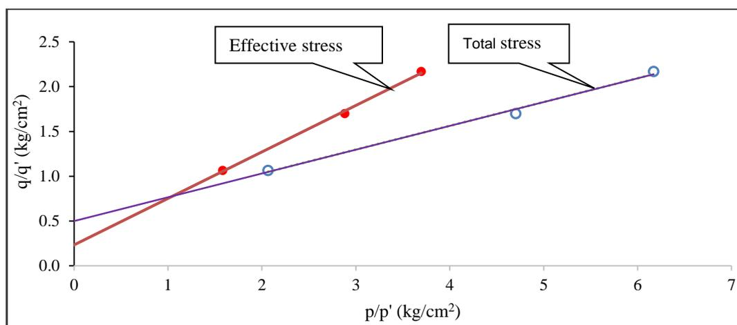
**Fig. 9.** 'p-q' plot with strength envelopes obtained at 20 % strain for sample no. 1.
