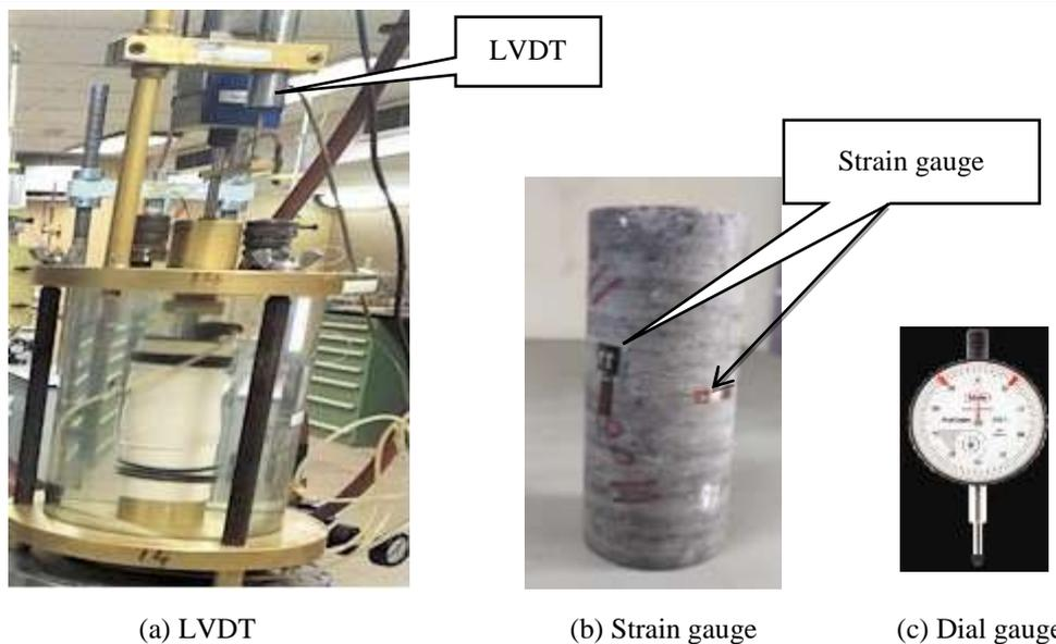
Fig. 3. Strain measuring instruments
