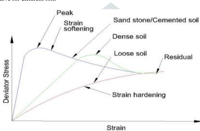
Fig. 2. Deviator stress- strain curve for different soil
