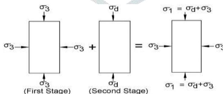
Fig. 6. Cylindrical specimen subjected to stresses in CU test
