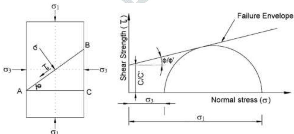
**Fig. 1.** Mohr's graphical representation of stresses
