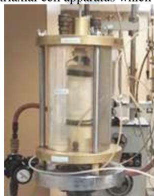
Fig. 4. Preparation of specimen in triaxial cell apparatus
