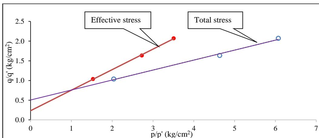
**Fig. 8.** 'p-q' plot with strength envelop obtained at 15 % strain for sample no. 1
