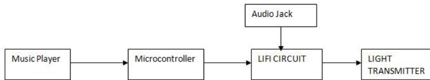
Fig 3.3. Transmitter of audio
