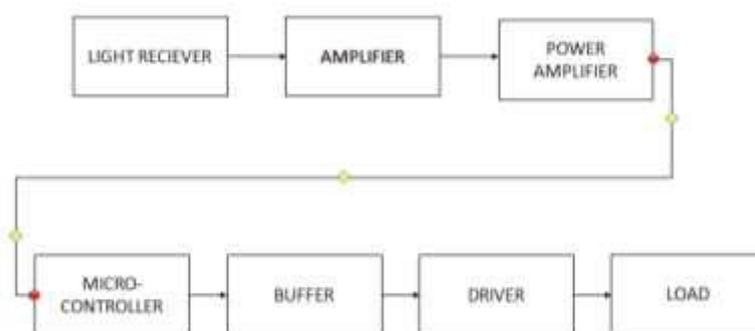
Fig 3.2. Receiver for device control
