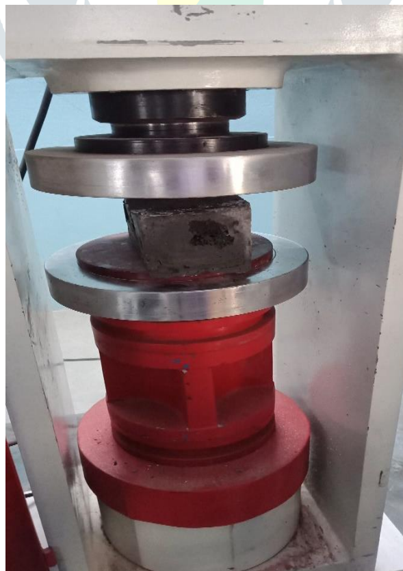
Compressive Strength Test of Plastic Brick
