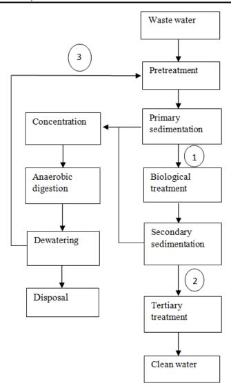
Fig 1: Wastewater treatment process.
