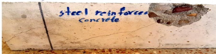
D) Fig 13. Typical fracture of steel RC
