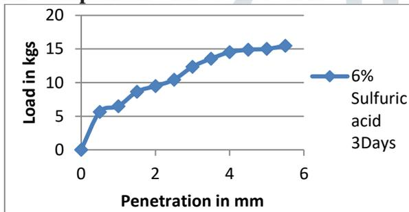
**Graph 4.1.2 Penetration Vs Load for Socked test**
