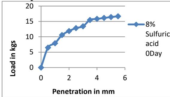
**Graph 4.1.1 Penetration Vs Load for Un-socked test**
