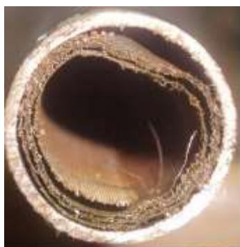
heat pipe with screen mesh wick
