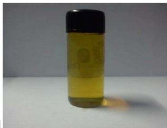
Silver nanofluid having average particle size around 20 nm
