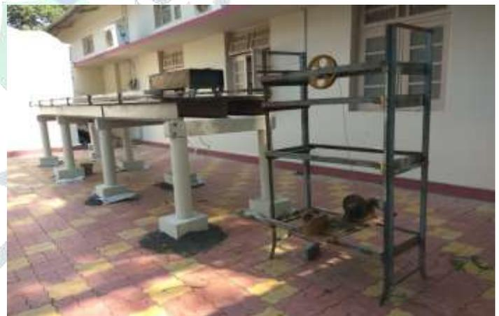
Fig.1: Composite Bridge Model
