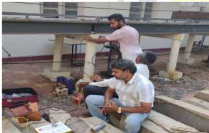
Fig.3: Ultrasonic Pulse Velocity Test
