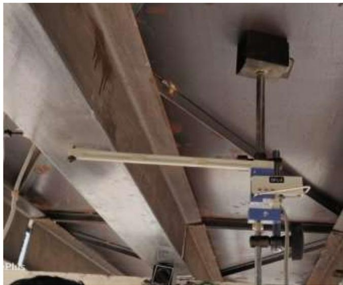
Fig.5: Deflectometer Connected to Longitudinal Girder
