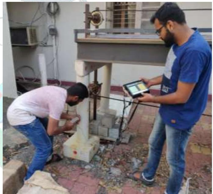
Fig.4: Rebound Hammer Test
