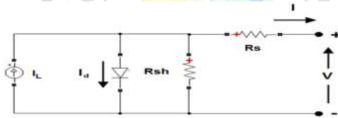
Figure 5 : PV model consider for the calculation of the photo current
