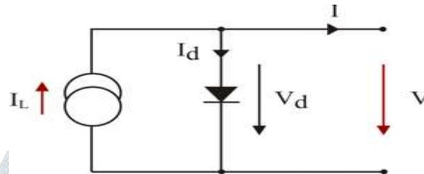
**Figure 2: Ideal diode model for PV cell.**
