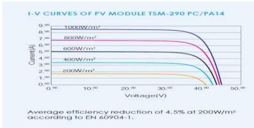
Figure 6 : I-V curves for the PV module for the irradiance parameter.
