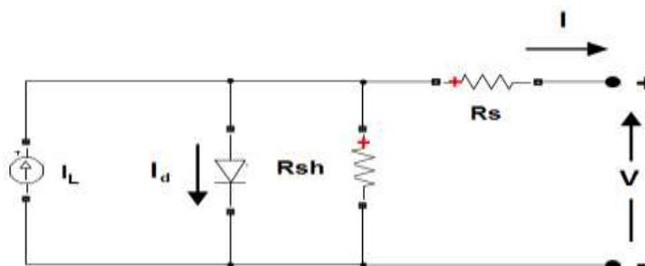
**Figure 3: Practical Single diode model for PV cell.**
