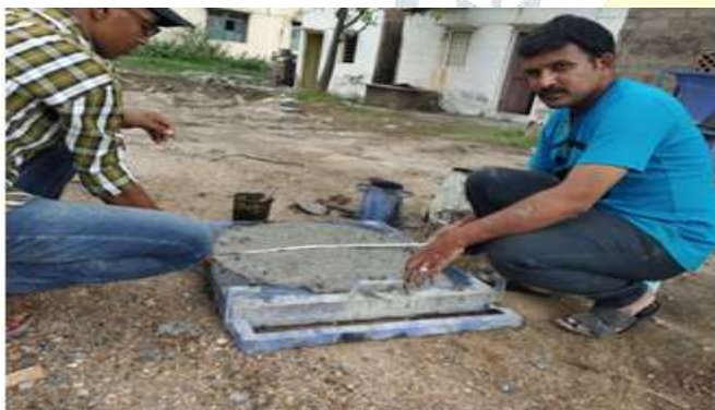
Fig 6.1 Slump flow testing
