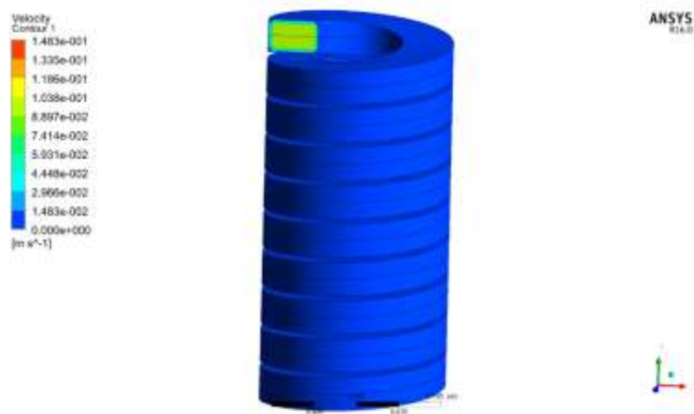
Fig 4. 8 velocity contour diagram (front view) for d= 0.05m
