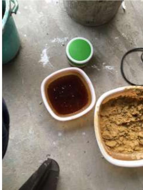
Gum, fuller's earth and baking soda ready for adding in the pulp
