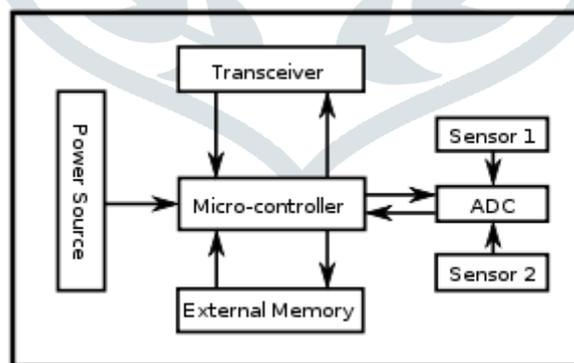
Fig. (1). The architecture of Wireless Sensor Node
