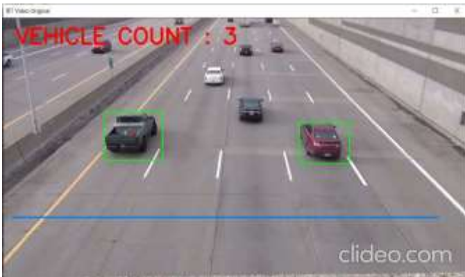
Fig 2. Real-Time Vehicle Counting using BackgroundSubtractorMOG Algorithm.
