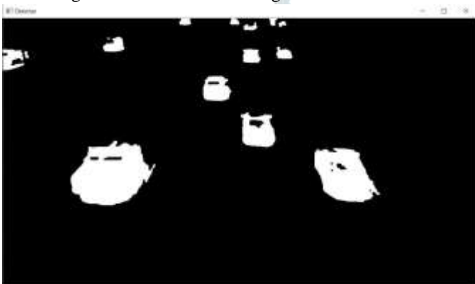
Fig 3. Real-Time Morphological Dilation and Contour Detection.
