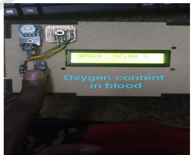
Fig.10. LCD Showing the Oxygen content value in blood
