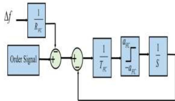
Fig 2. Dynamic Model of the Fuel Cell
