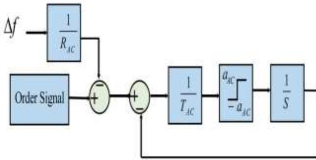
Figure 3. Dynamic Model of the Electrolyzer
