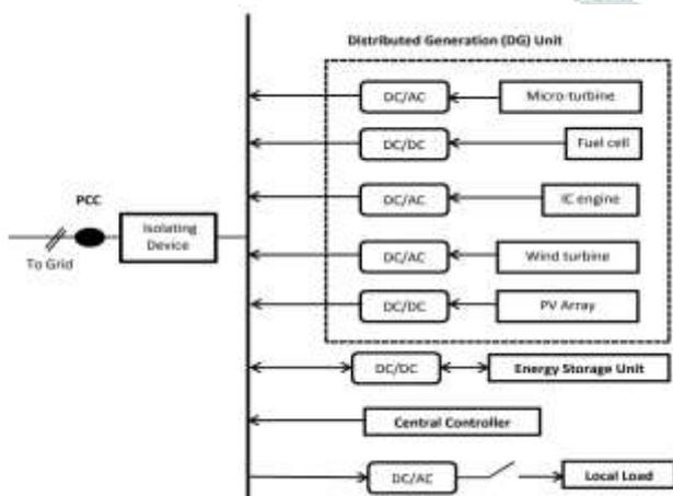
Fig.1. Generalized microgrid structure
