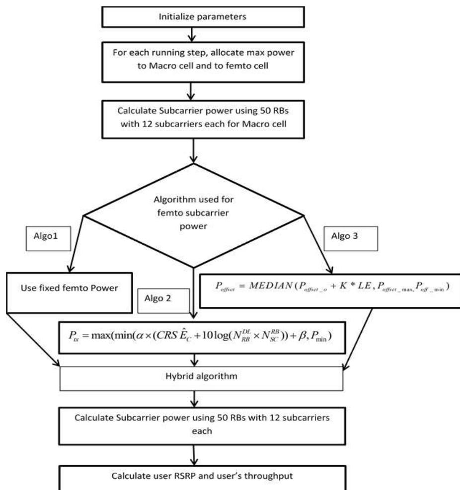
Figure 7: Flowchart for Femto power calculation and throughput calculation
