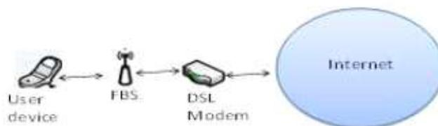
Figure 2: User device connected to an operator's core network in a femtocell
