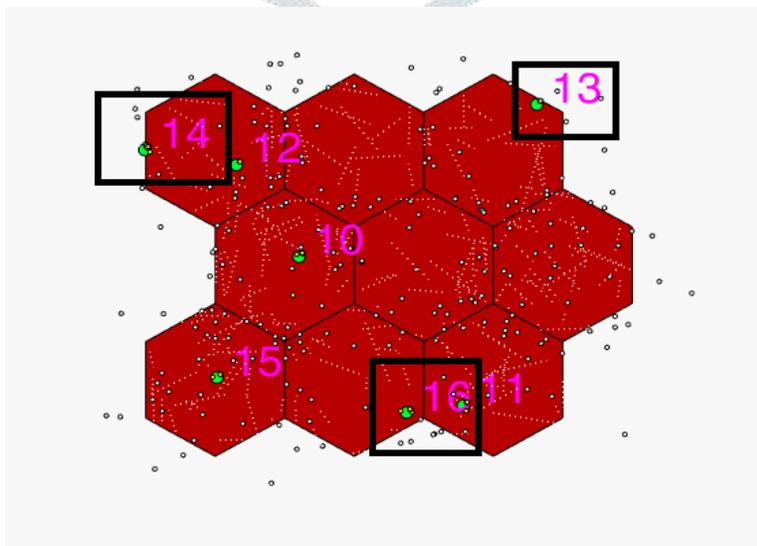
Figure 10: Image showing femto cells away from macro cell centers
