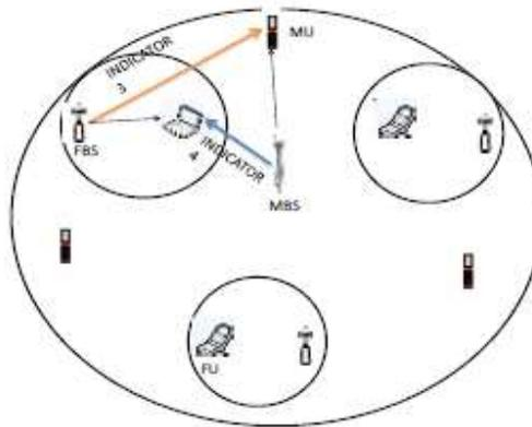
Figure 5: A scenario showing cross-tier interference between FBSs and MBSs [1]
