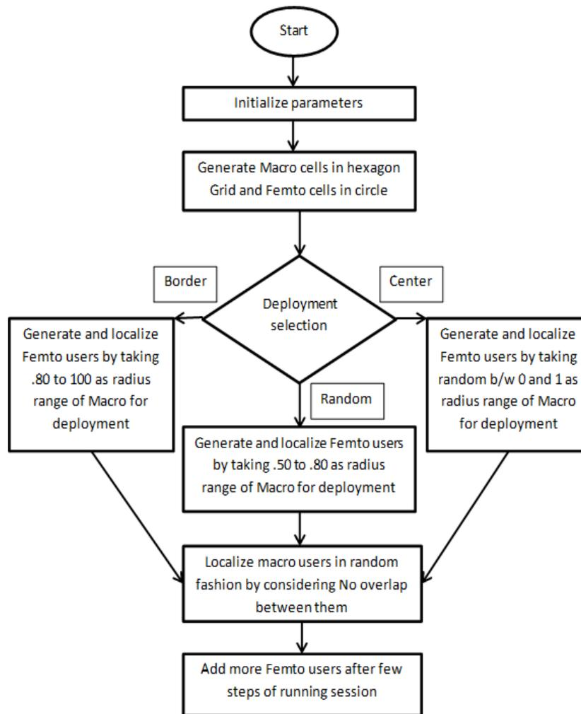
Figure 6: Flowchart for initial random deployment of Macro and Femto cells and users
