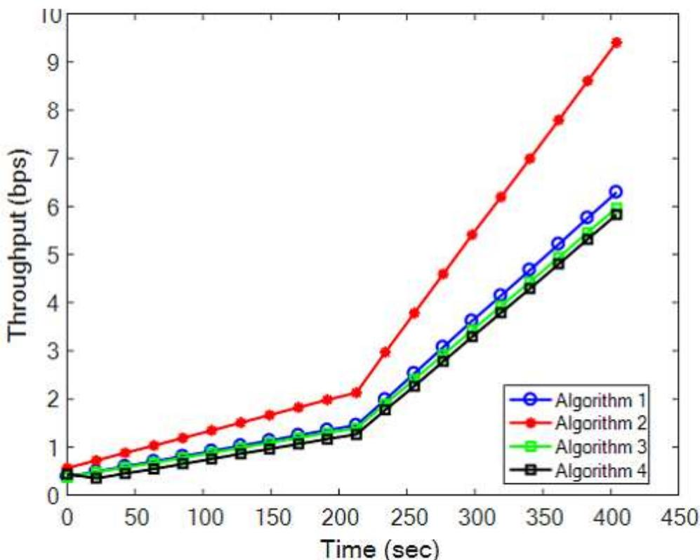
Figure 11: Achieved throughput using all four algorithms for femto cell 10
