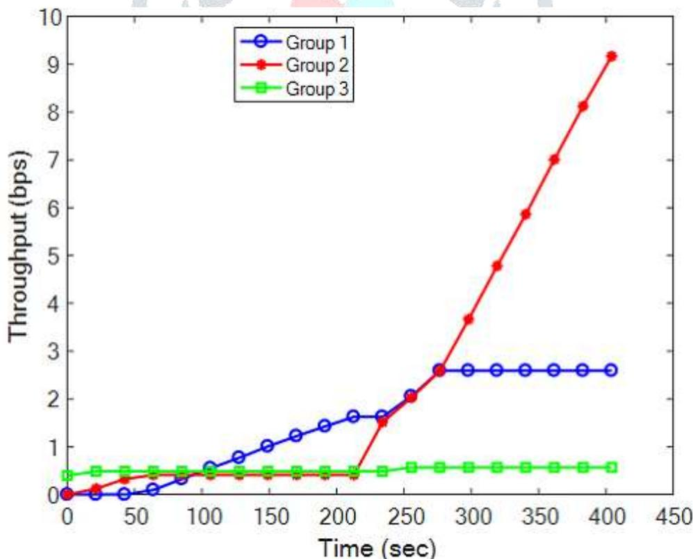
Figure 12: Groupwise achieved throughput for cell 10 using hybrid algorithm
