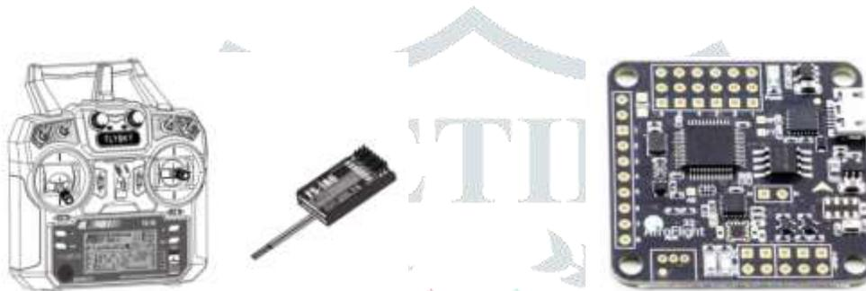
Fig6: Transmitter and Receiver Used in Tricopter      Fig7: Flight Control Card used in Tricopter
