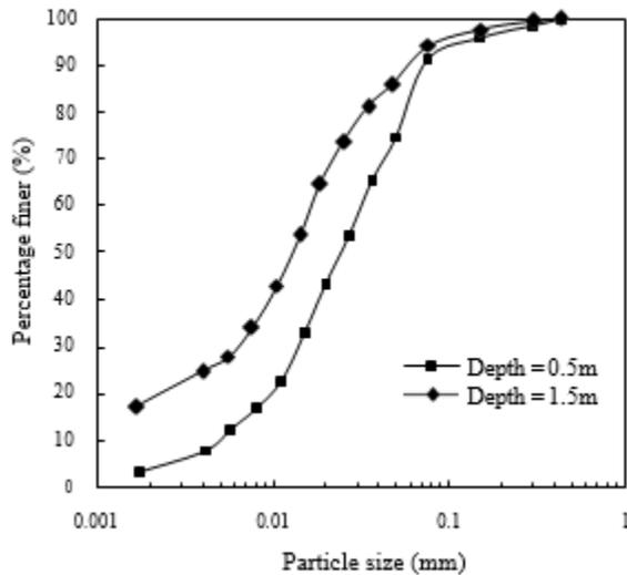
Figure 3. Particle size distribution curve for Bemina soil.
