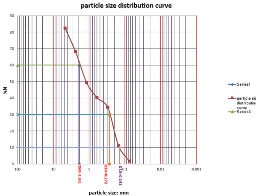
Figure 1: Particle Size Distribution Curve for soil sample collected at Phagwara
