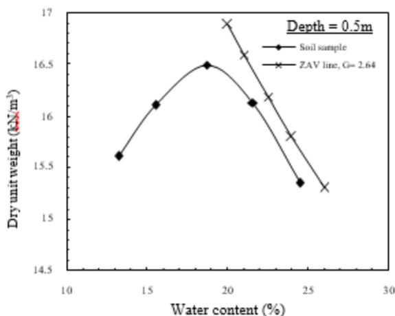
Figure 4. Compaction curve of Bemina soil.
