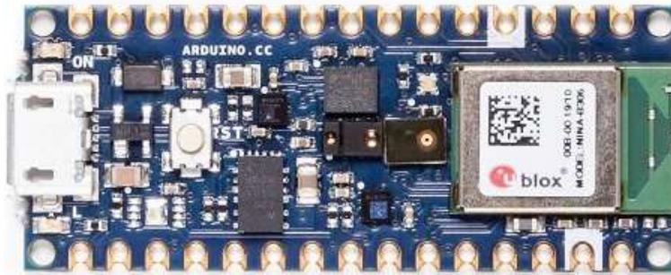
The Nano 33 BLE Sense is Arduino's 3.3 V AI enabled board in the smallest available form factor.
