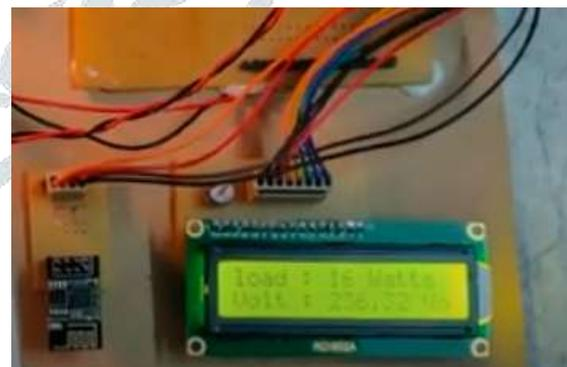
Fig: 5 voltage, load monitoring on LCD display
