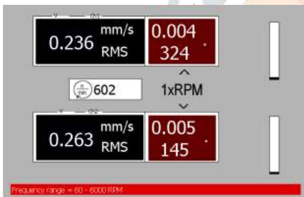
Figure 20. Vibrometer reading at 600 rpm in Horizontal Plane
