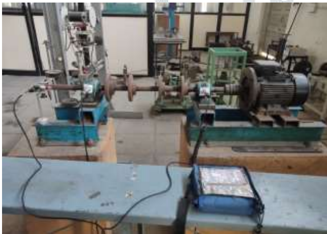
Figure 4. Sensors in Horizontal Direction
