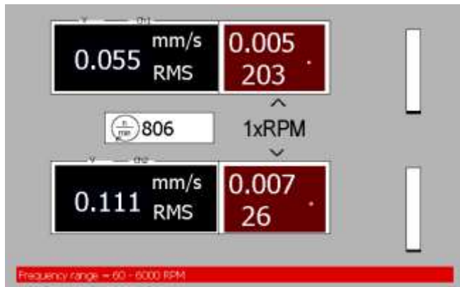
Figure 16. Vibrometer reading at 800 rpm in Axial Plane
