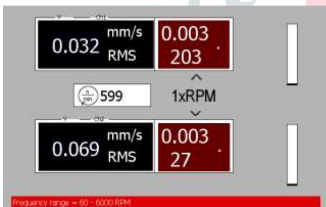
Figure 28. Vibrometer reading at 600 rpm in Axial Plane
