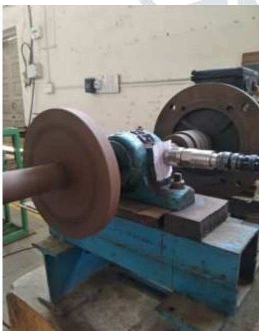
Figure 6. Accelerometer in Horizontal plane
