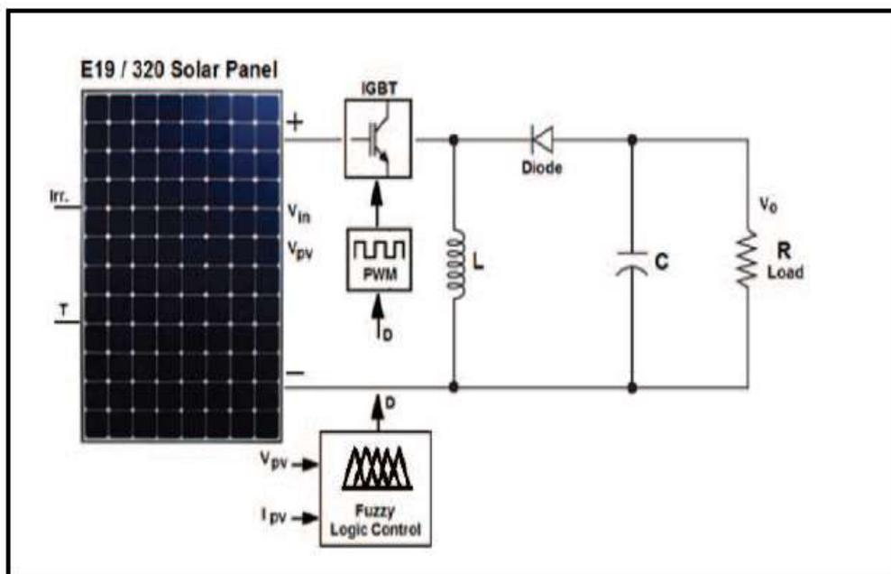
Fig.2. MPPT Tracking using fuzzy logic controller [2]
