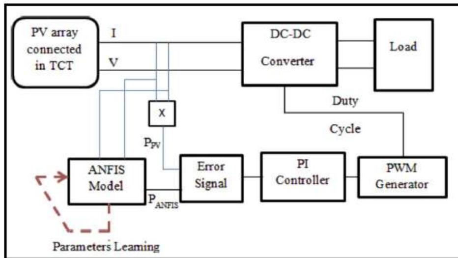
Fig.3. Block diagram of ANFIS controller for MPPT tracking [3]
