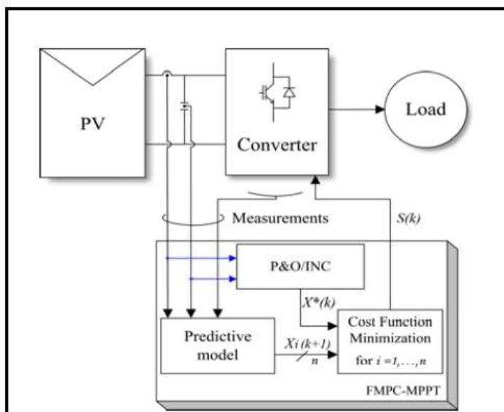
Fig.4. FMPC based MPPT tracking approach block diagram [4]
