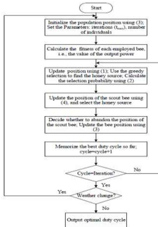
Fig.7. MABC MPPT algorithm block diagram
