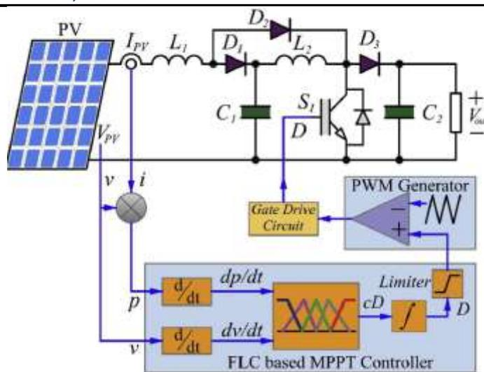
Fig.1. MPPT converter topology using Fuzzy logic controller [1]
