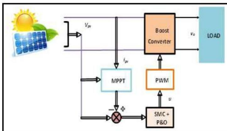
Fig.5. Block diagram of P & O MPPT approach [6]
