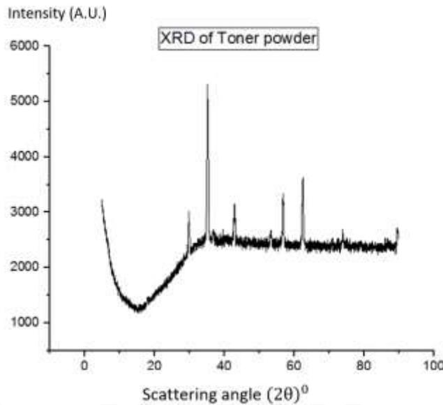
**Figure 1:** XRD pattern for toner powder sample at room temperature 25°C
