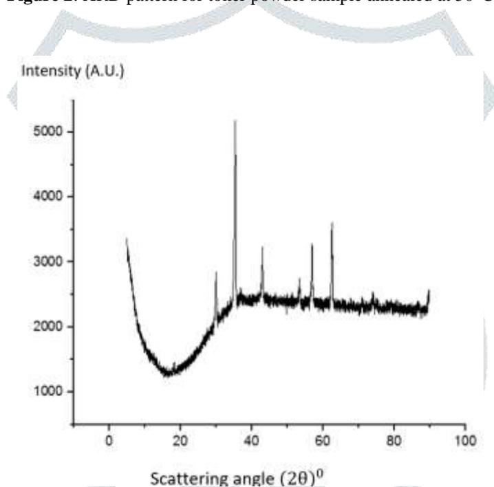
Figure 3: XRD pattern for toner powder sample annealed at 100°C
