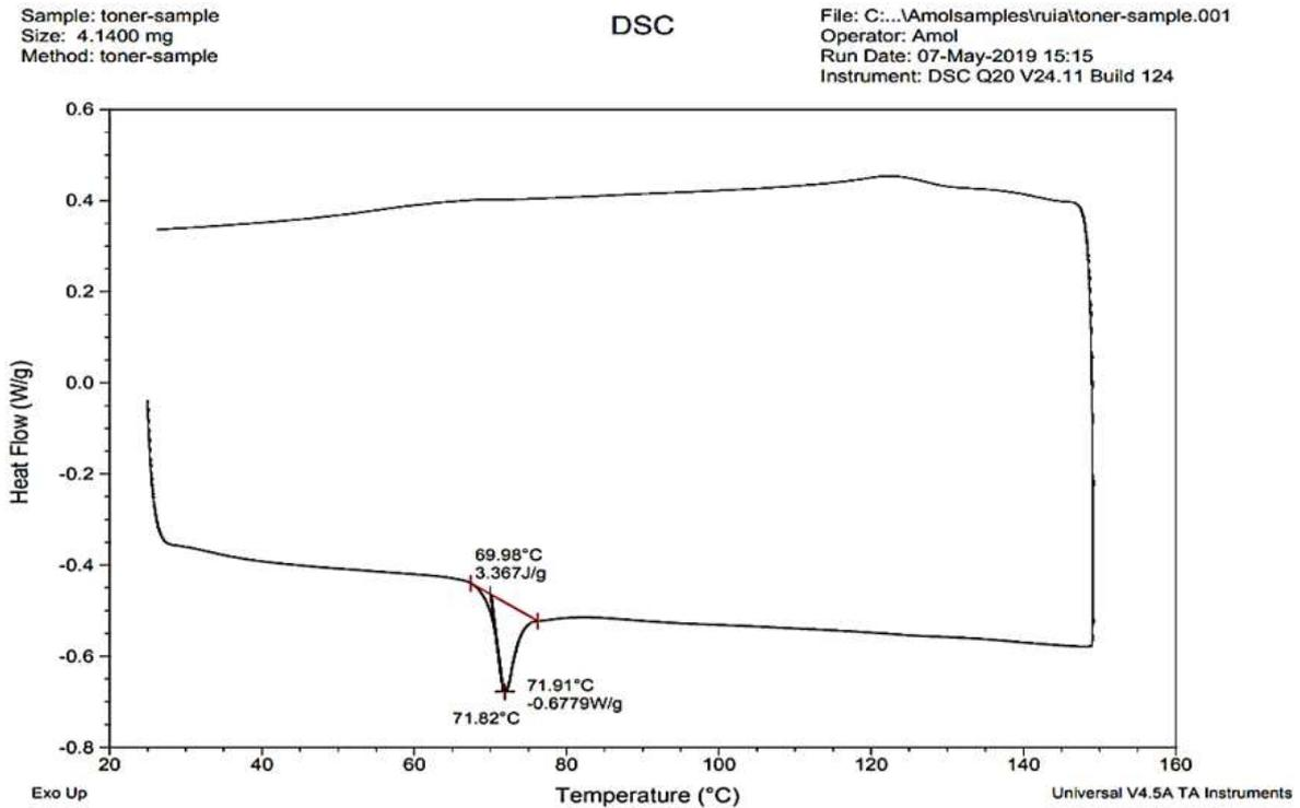
Figure 9: Heating run of the toner sample (IIT-B laboratory)
