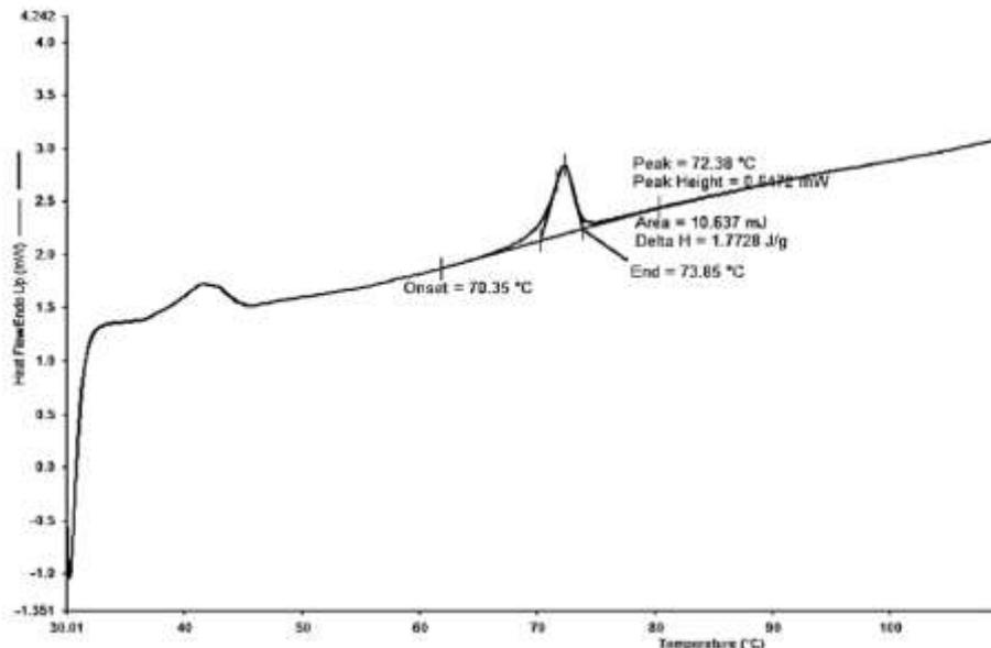
Figure 7: Heating run of the toner sample (ICT laboratory, Mumbai)
