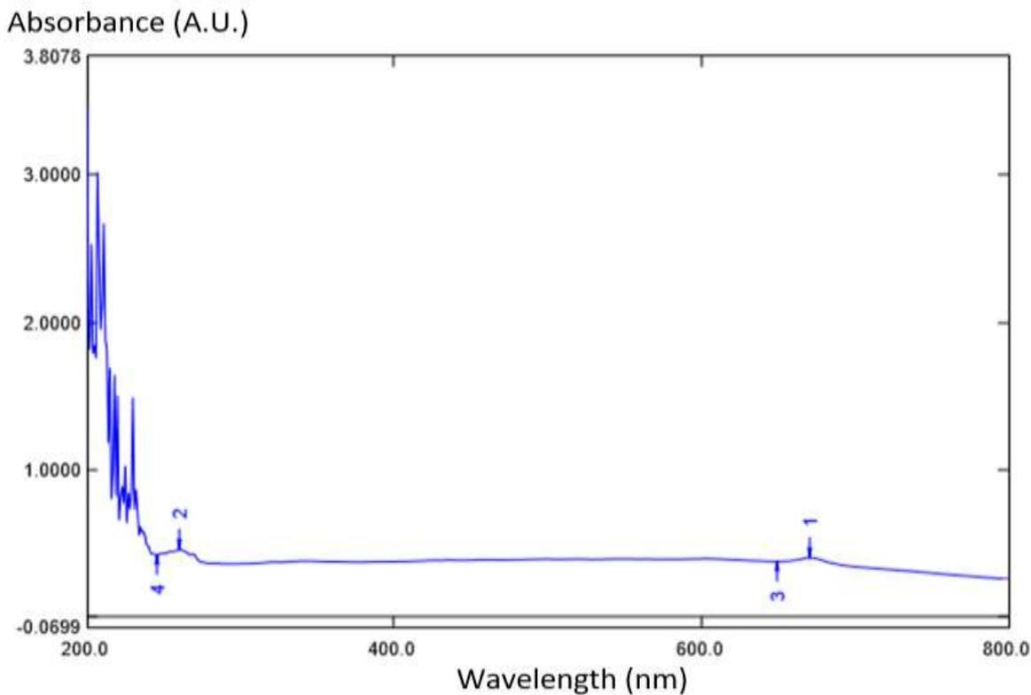
Figure 4: UV-Vis spectrum of toner sample powder at RT (wavelength-200nm-800nm)
