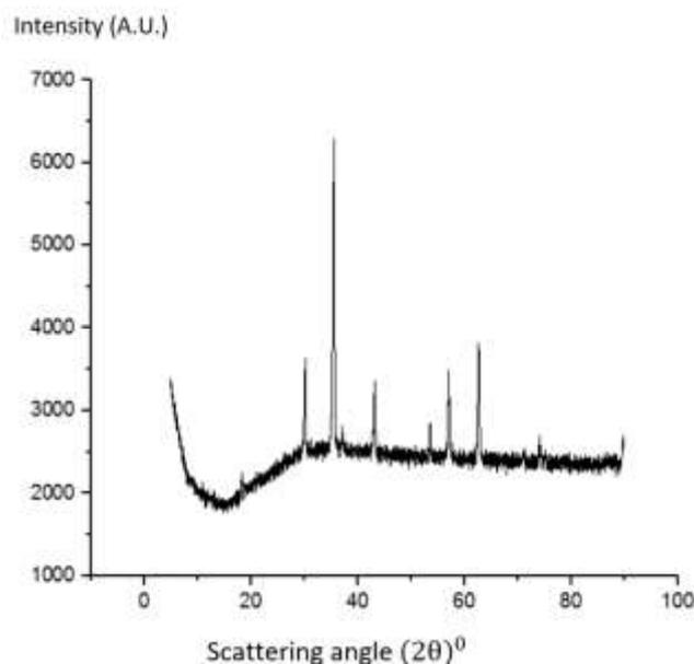
Figure 2: XRD pattern for toner powder sample annealed at 50°C
