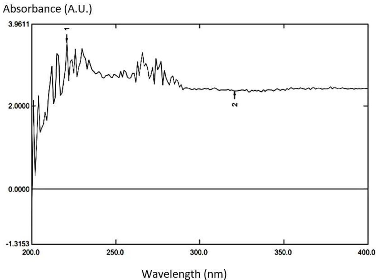
Figure 5: UV spectrum of the toner sample at RT (wavelength-200nm-400nm)
