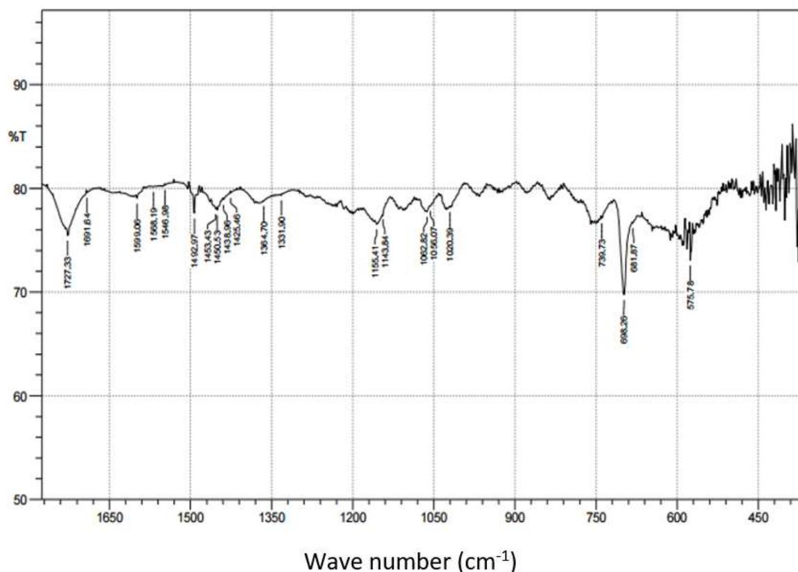
Figure 6: FTIR spectroscopy of the toner sample powder.
