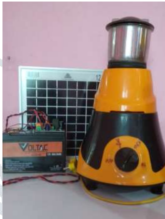
Fig: Solar operated mixer grinder
