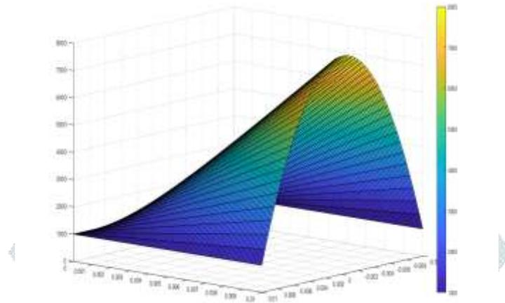
Fig 8. Temperature Variations Due To Electrode Droplet On The Work Piece Surface
