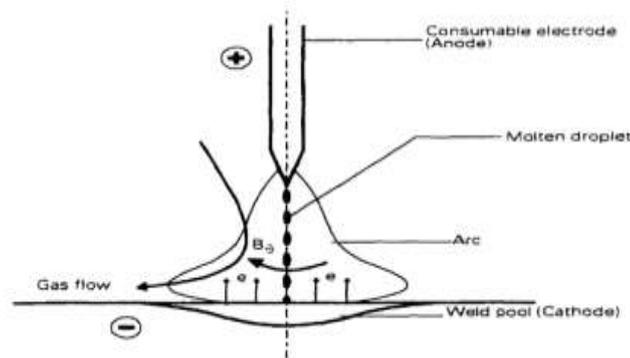
Fig 2 Schematic of Welding Arc (GMAW)
