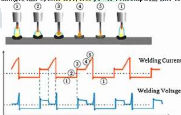
**Fig 1.** Metal Transfer Process, Current and Voltage Waveforms of Cold Metal Transfer Welding
