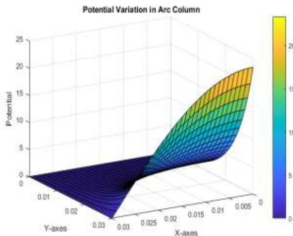
Fig 7. Potential Variations Due To Electrode Droplet In Arc Region
