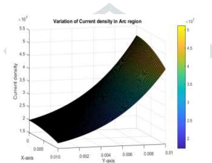
Fig 6. Variation of Current Density in Arc Region
