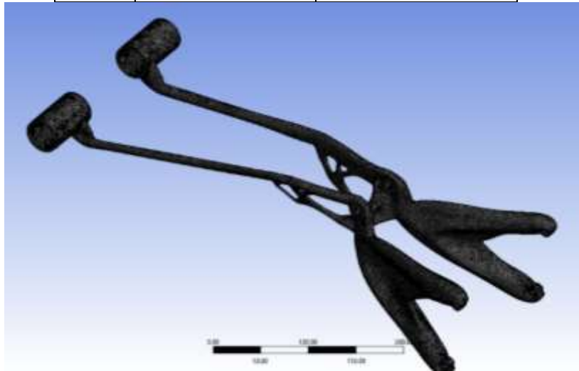
Figure 12. Isometric view of final meshed swingarm.
