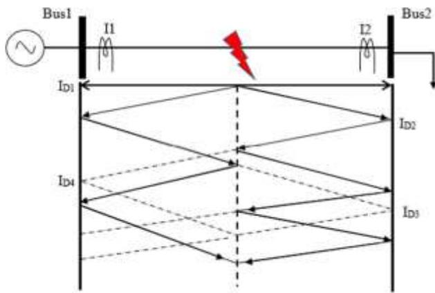
Fig. 1 Traveling wave phenomenon
