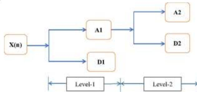
Fig. 2 Discrete wavelet transform-multi-resolution analysis
