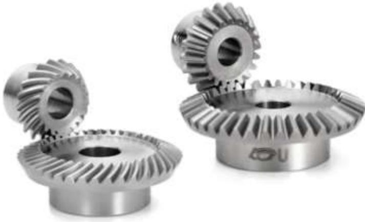
Bevel gears are [gears](#) where the axes of the two [shafts](#) intersect and the [tooth](#)-bearing faces of the gears themselves are conically shaped. Bevel gears are most often mounted on shafts that are 90 degrees apart, but can be designed to work at other angles as well. The pitch surface of bevel gears is a [cone](#)
