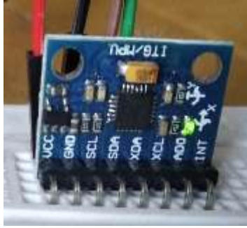
Fig.(e) Accelerometer MPU6050
