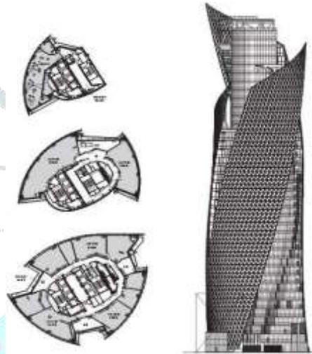
Fig. 7 The Mode Gakuen Spiral Tower - Plan and cross-section common support system is the diagrid system. In this system, lateral displacements increase as the geometrical form deviates from the classical rectangular cuboid shape. As the degree of oscillation of the form increases, the diagonal angle deviates from the optimal value, which in turn reduces the lateral stiffness of the building.
