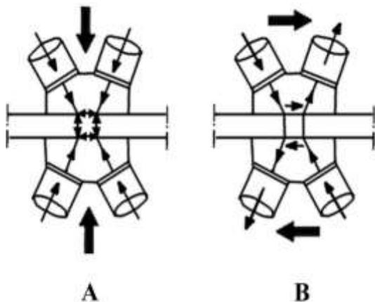
Fig. 2 The diagrid structural system node: A) under vertical
