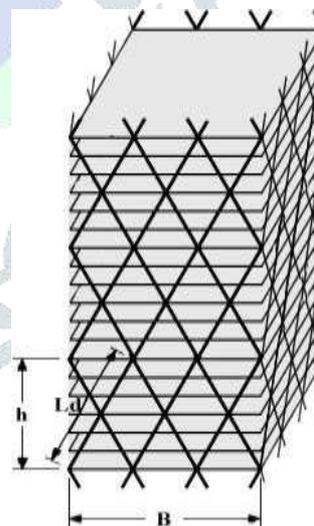
Fig. 3 Typical diagrid module
