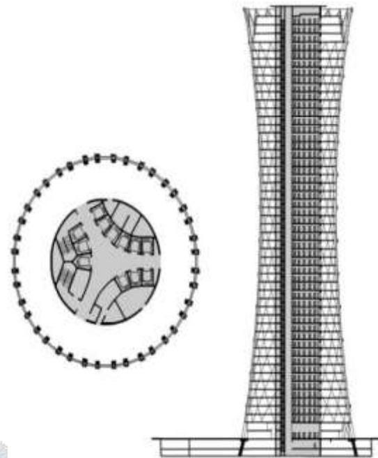
Fig. 9 The Tornado Tower – Plan and cross-section
