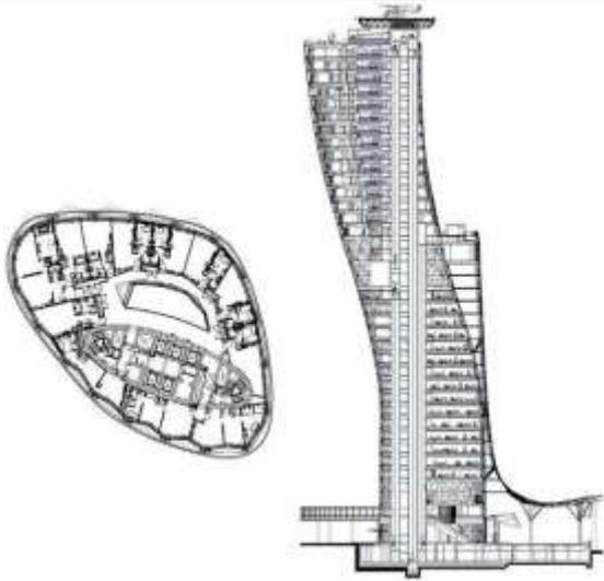
Fig. 10 The Capital Gate Tower – Plan and cross-section
