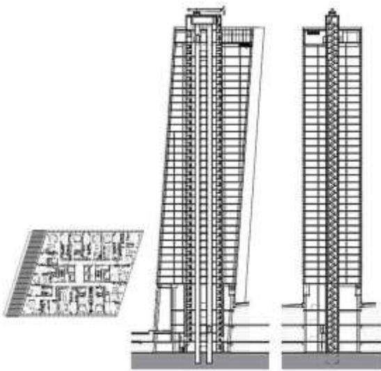
Fig. 5 The Veer Towers - Plan and cross-section
