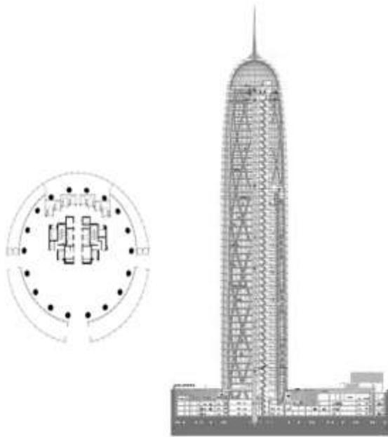
Fig. 8 The Doha Tower – Plan and cross-section
