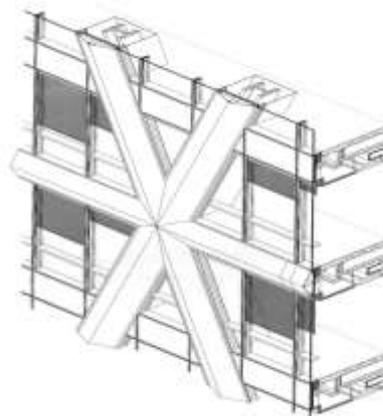
Fig. 1 Detail of the diagrid system
