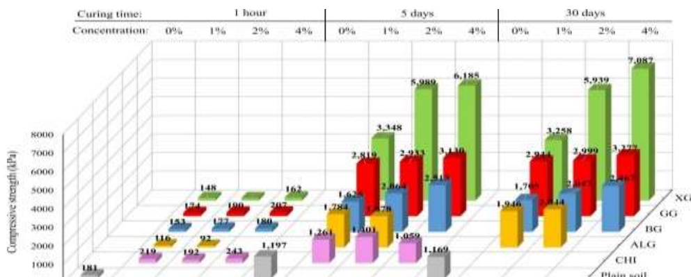
Figure 6. Change in compressive strength under the influence of time, biopolymer-type, and biopolymer concentrations. (Adopted from Antonio Soldo et al., 2020)
