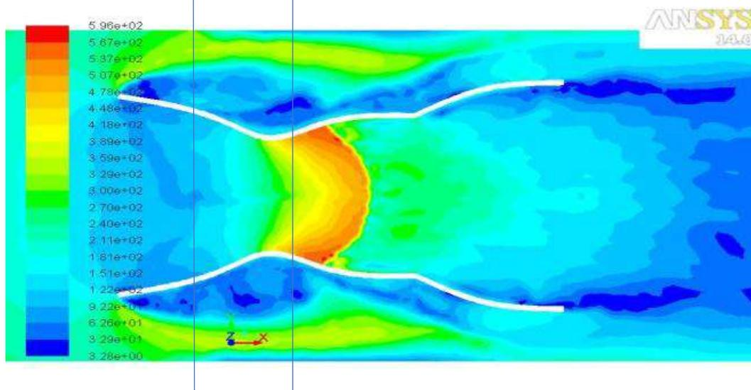
**Figure 2:** velocity variation at pipe and nozzle (ref. 2).
