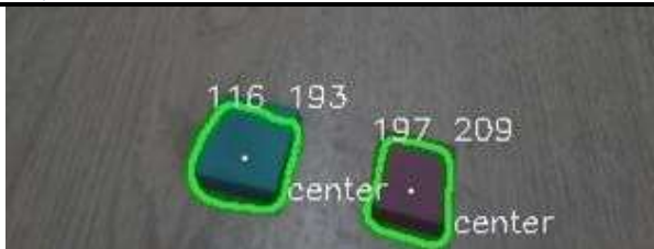
Fig:3 The object detection and the center of the objects in the image
