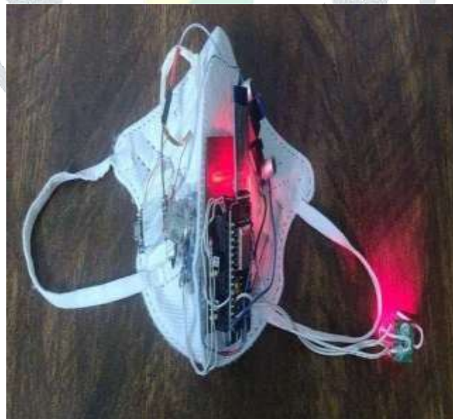
Figure 8: Various sensors, oximeter module and UV led interfacing with NodeMCU , integrated with N95 mask.
