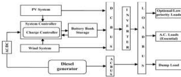
Fig. 1. Basic component of solar–wind hybrid renewable energy system.
