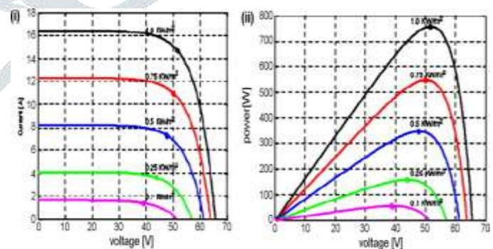
Fig. 2. (i) I–V characteristics of PV module and (ii) P–V characteristics of PV module.
