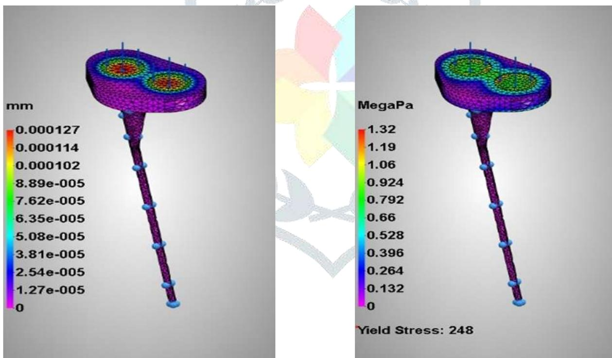
Figure 4 Static structural, Displacement and Von- Misses stress (60 kg)
