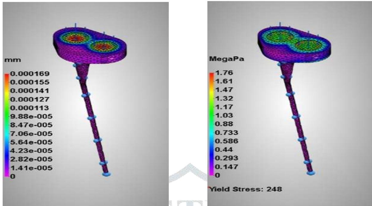
Figure 5 Static structural, Displacement and Von- Misses stress (80 kg)
