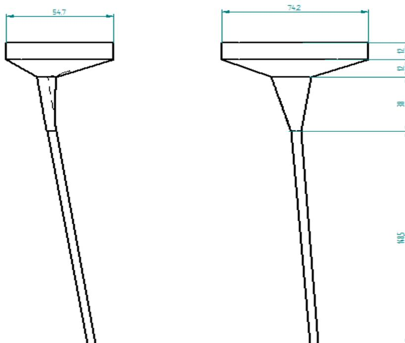
Figure 3 View of tibia intramedullary implant (Dimensions in mm)
