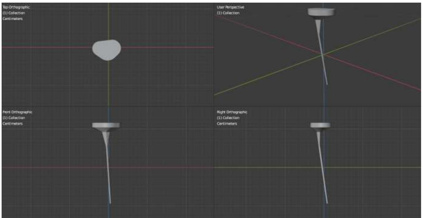
Figure 2 CAD model of tibia intramedullary implant
