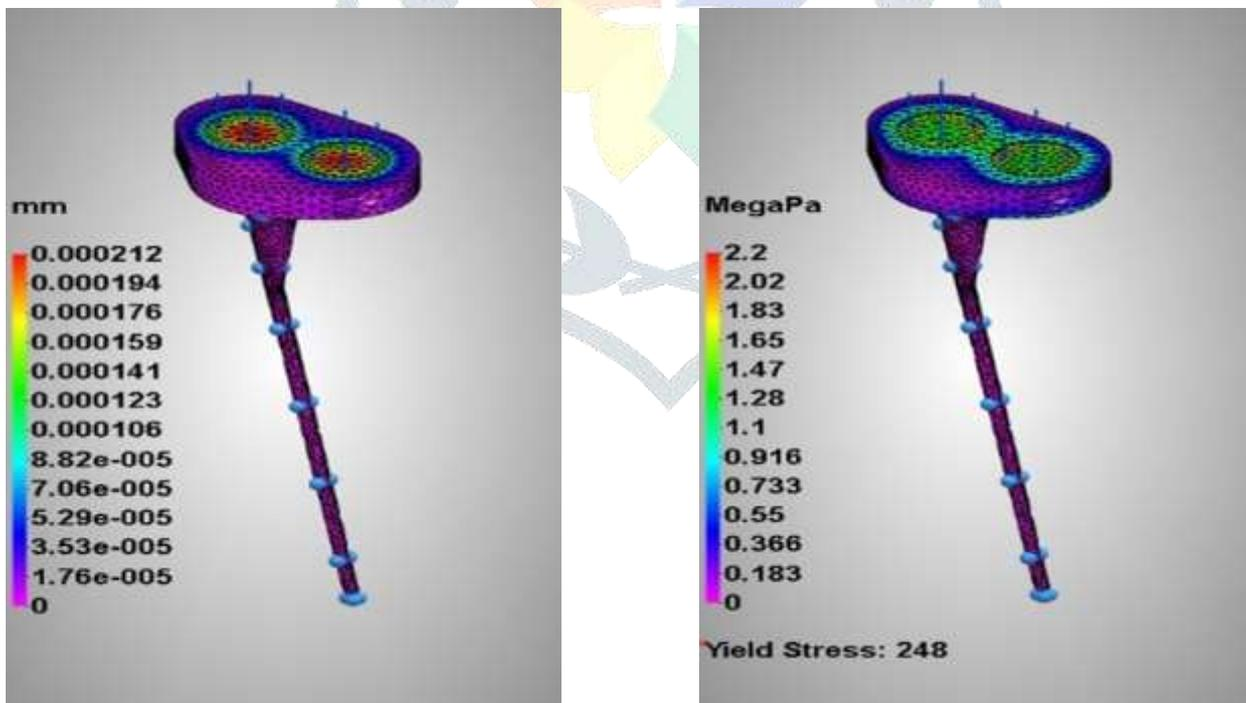
Figure 6 Static structural, Displacement and Von- Misses stress (100 kg)
