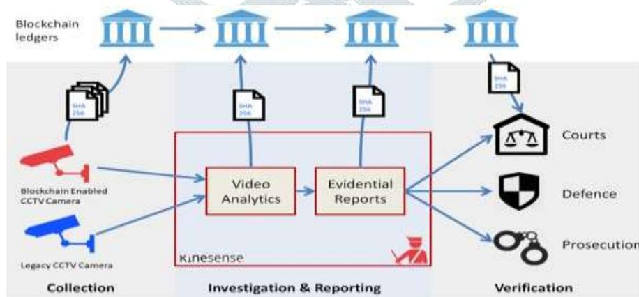
Figure 3: Blockchain for Chain of Management (CoM) in CCTV
