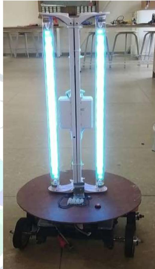
Figure 8: Final UV disinfection robot
