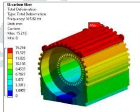
Fig. Mode shape 1 with fundamental frequency 315.62 Hz
