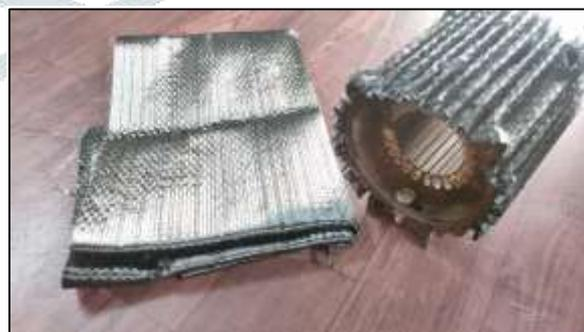
Fig. Motor housing with carbon fiber
