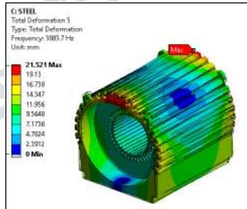
Fig. Mode shape 5 with natural frequency of 3883.7 Hz
