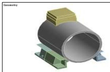
Fig Geometry of motor casing
