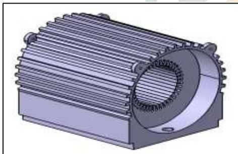
Fig. Motor bracket cad model
