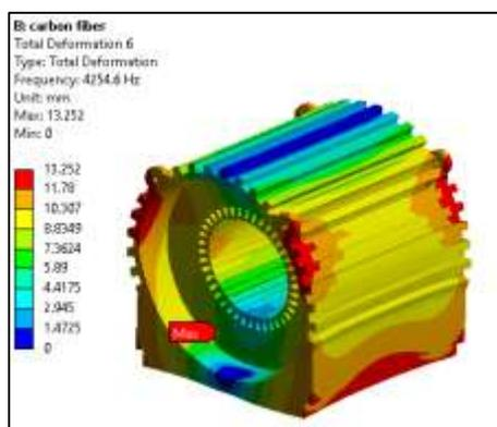
Fig. Mode shape 6 with natural frequency 4254.6 Hz
