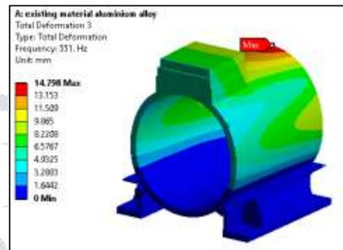
Fig. Mode shape 3 with fundamental frequency 551 Hz
