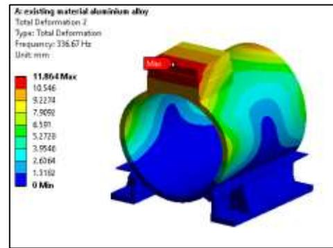
Fig. Mode shape 2 with fundamental frequency 336.67Hz
