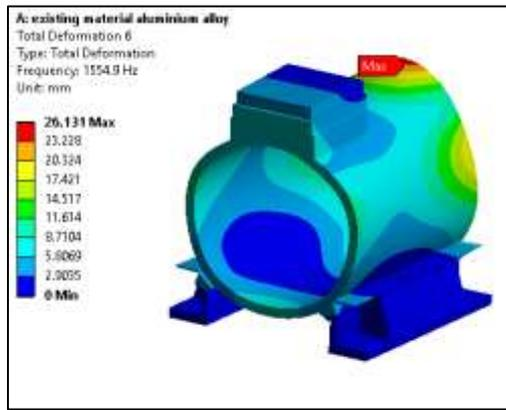
Fig. Mode shape 5 with fundamental frequency 1554.9 Hz
