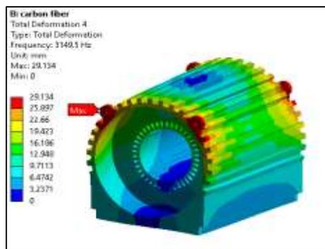
Fig. Mode shape 4 with natural frequency 3149.5 Hz
