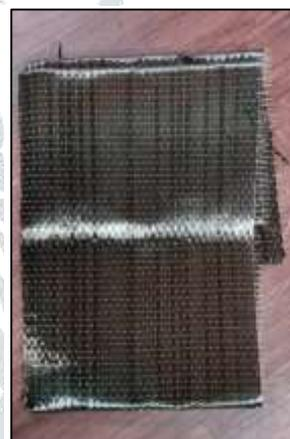
Fig. Sheet of carbon fiber
