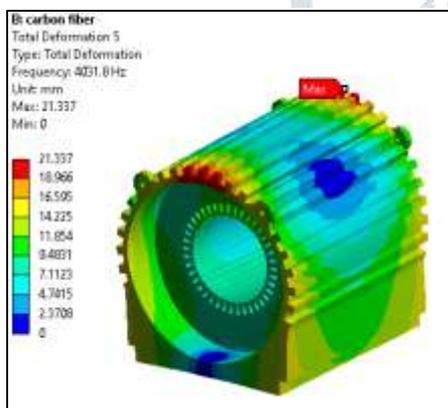
Fig. Mode shape 5 with natural frequency 4031.8 Hz
