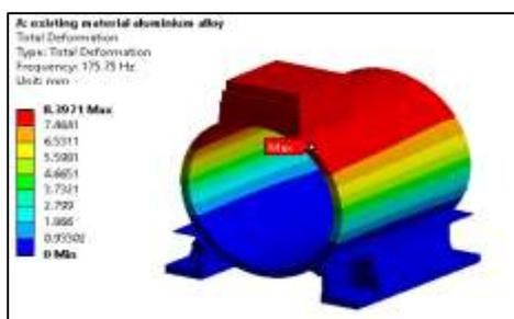
Fig. Mode shape 1 with fundamental frequency 175.75Hz
