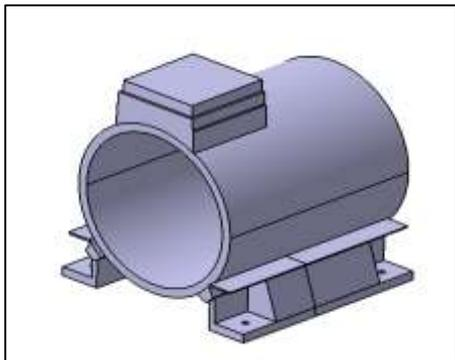
Fig.1 CATIA model of motor casing
