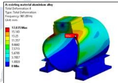
Fig. Mode shape 4 with fundamental frequency 961.09 Hz
