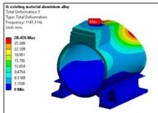
Fig. Mode shape 5 with fundamental frequency 1141.3 Hz
