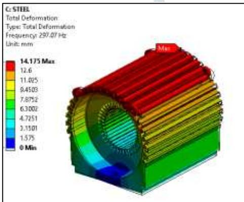
Fig. Mode shape 1 with fundamental frequency of 297.07 Hz
