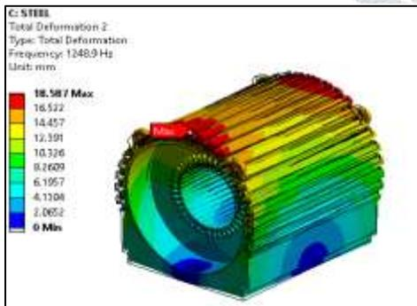
Fig. Mode shape 2 with natural frequency of 1248.9 Hz
