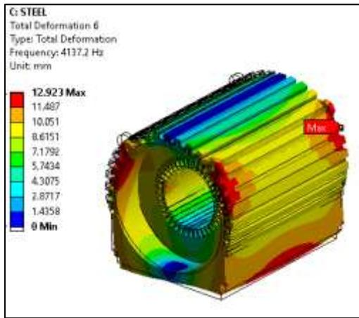
Fig. Mode shape 6 with natural frequency of 4137.2 Hz
