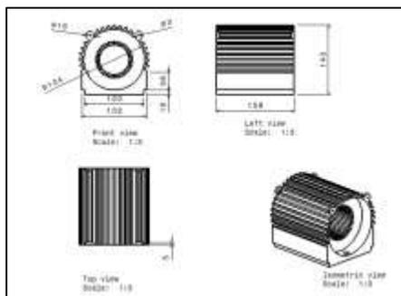
Fig. Drafting of motor casing
