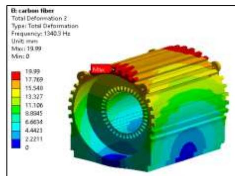
Fig. Mode shape 2 with natural frequency 1340.3 Hz
