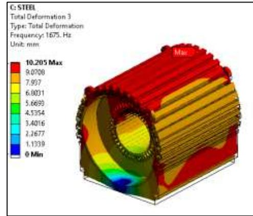
Fig. Mode shape 3 with natural frequency of 1675 Hz
