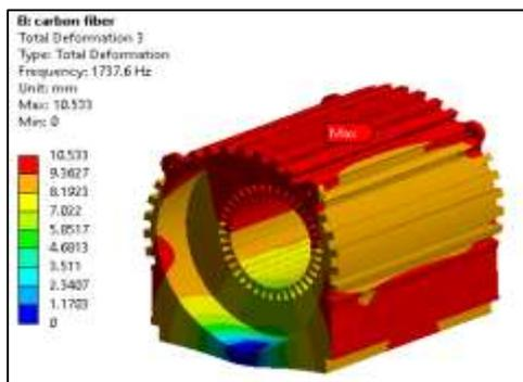
Fig. Mode shape 3 with natural frequency 1737.6 Hz
