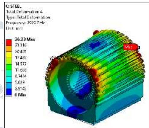
Fig. Mode shape 4 with natural frequency of 2929.7 Hz
